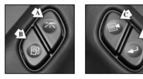
A (**Trip Information**): This button will display the odometer, personal trip odometer, business trip odometer, hourmeter, annual log and the timer.
