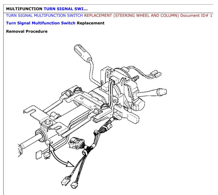
**Important:** The turn signal multifunction switch and Inflatable restraint steering wheel module coil ar serviced as an assembly.
