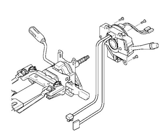
4. Remove the turn signal multifunction switch bolts.5. Slide the multifunction turn signal switch off of the steering column.
