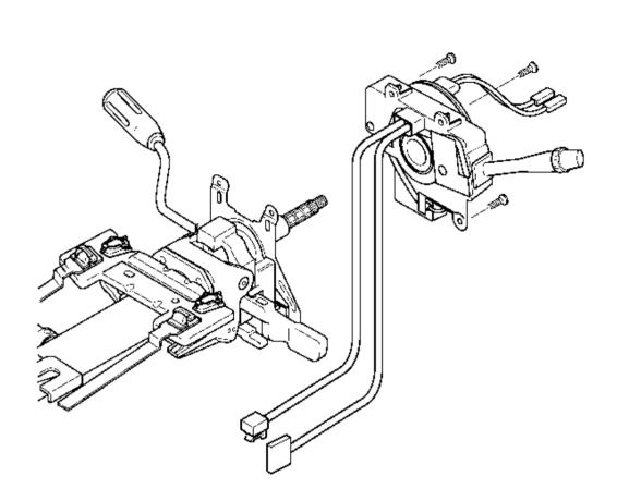
**Important:** A new multifunction turn signal switch will come precentered with a centering tab attache NOT remove the centering tab until installation is complete. Failure to follow procedure will cause a misalignment of the multifunction turn signal switch and centering will be required.
