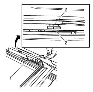
**Notice:** When manually repositioning the sunroof module guide mechanisms, push only on the guide shoes in order to eliminate the risk of damage to the components.
