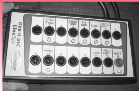
FIGURE 12-20 A break-out box (BOB) used to access the BUS terminals while using a scan tool to activate the modules. This break-out box is equipped with LEDs that light when circuits are active.
