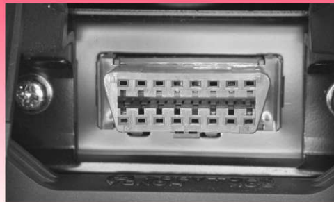
FIGURE 12-23 A DLC from a pre-CAN Acura. It shows terminals in cavities 4, 5 (grounds), 7, 10, 14, and 16 (B+).
