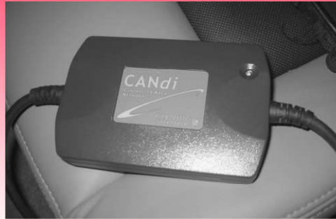
FIGURE 12-11 A CANDi module will flash the green LED rapidly if communication is detected.
