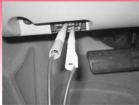
FIGURE 12-29 Use front-probe terminals to access the data link connector. Always follow the specified back-probe and front-probe procedures as found in service information.
