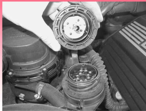
FIGURE 12-22 A typical 38-cavity diagnostic connector as found on many BMW and Mercedes vehicles under the hood. The use of a break-out box (BOB) connected to this connector can often be used to gain access to module BUS information.
